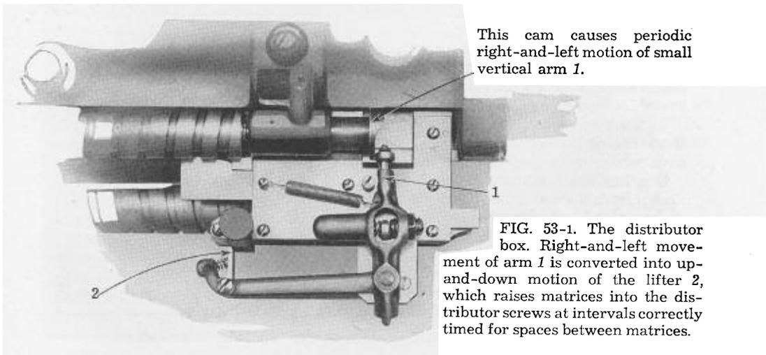
This cam causes periodic right-and-left motion of small vertical arm 1.
