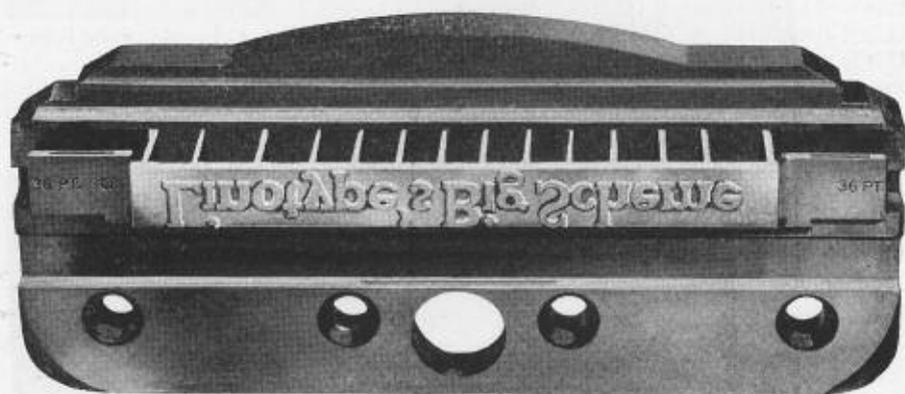
FIG. 32-1. Display mold.
