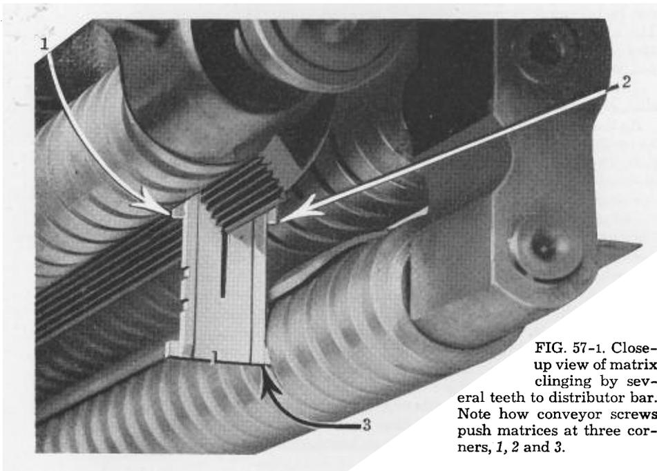
FIG. 57-1. Close-up view of matrix clinging by several teeth to distributor bar. Note how conveyor screws push matrices at three corners, 1, 2 and 3.
