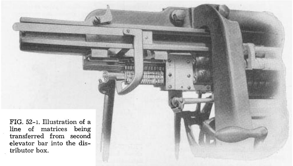
FIG. 52-1. Illustration of a line of matrices being transferred from second elevator bar into the distributor box.
