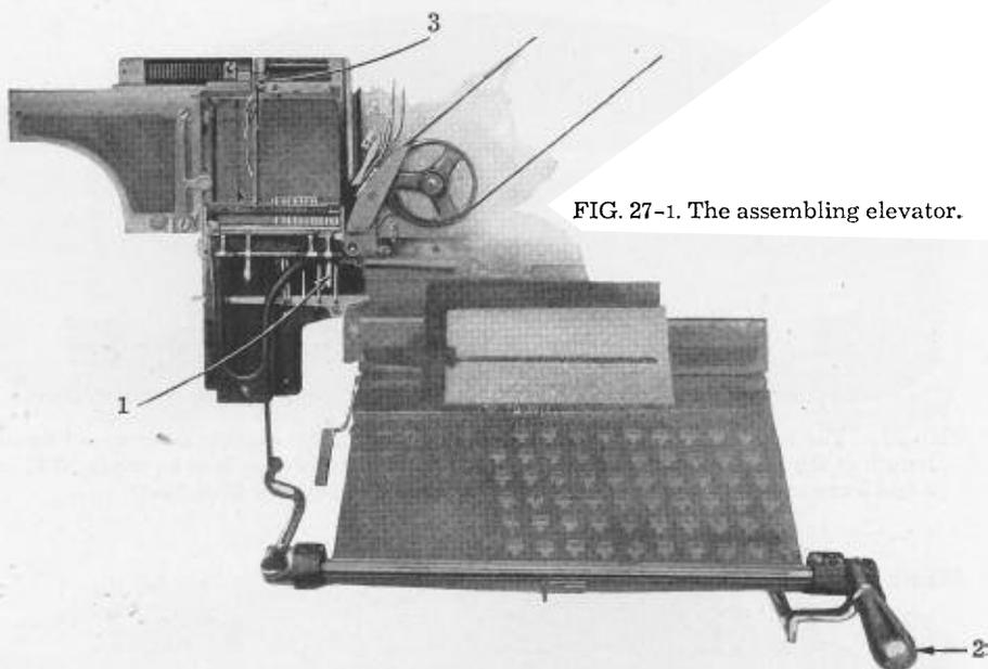
FIG. 27-1. The assembling elevator.
