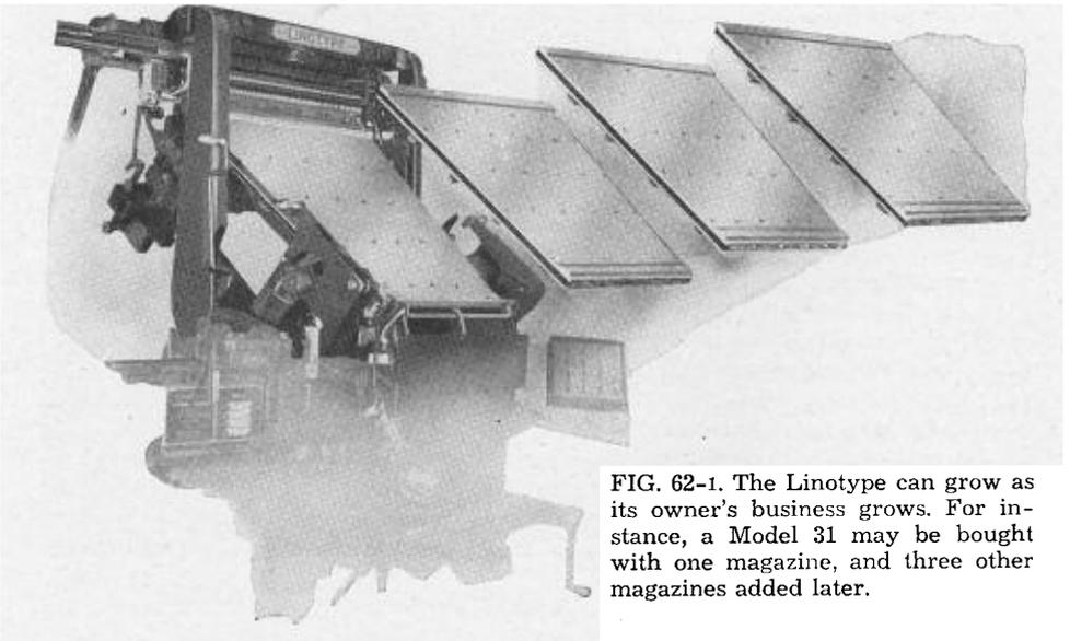
FIG. 62-1. The Linotype can grow as its owner's business grows. For instance, a Model 31 may be bought with one magazine, and three other magazines added later.
