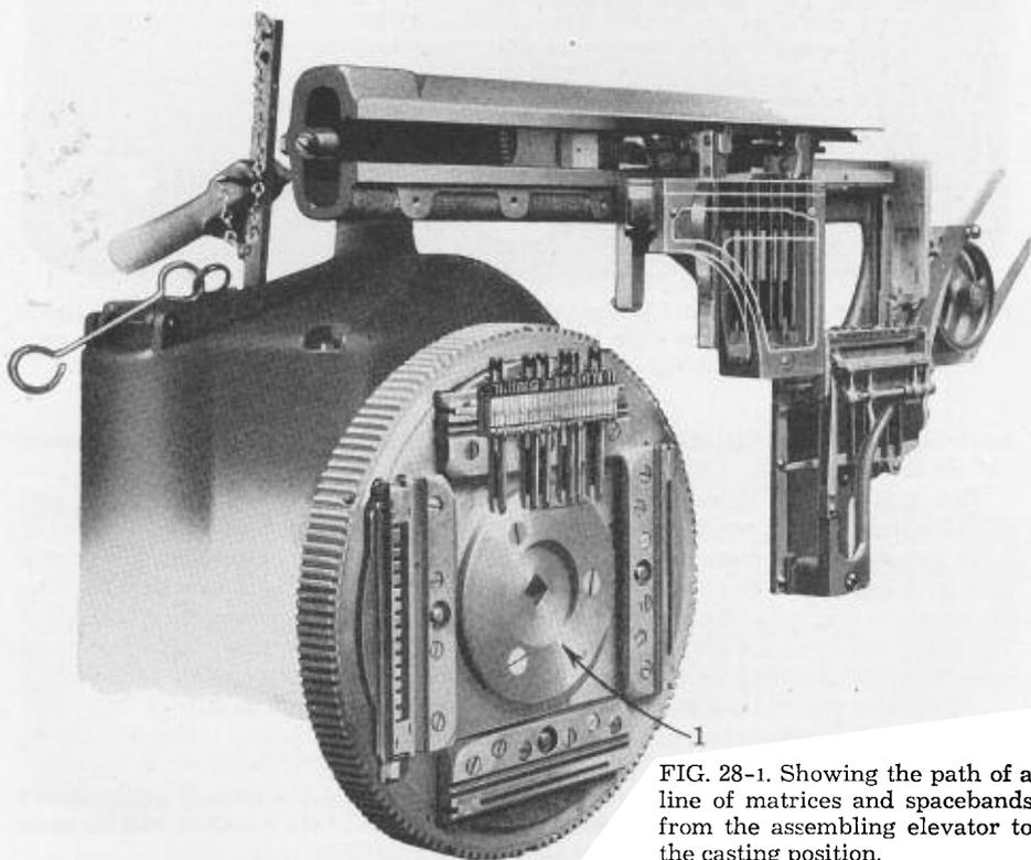
FIG. 28-1. Showing the path of a line of matrices and spacebands from the assembling elevator to the casting position.
