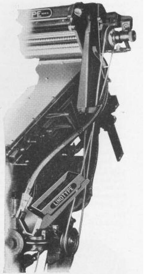
FIG. 58-1. View of the sorts stacker for pi matrices.
