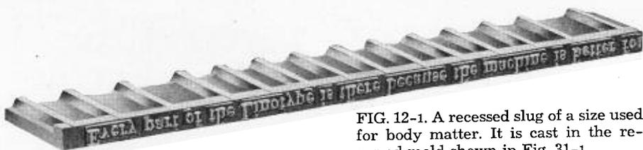
FIG. 12-1. A recessed slug of a size used for body matter. It is cast in the recessed mold shown in Fig. 31-1.
