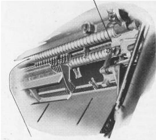
Each matrix is moved along by these screws to a point at which the corresponding teeth on the bar are cut away and cease to support it. It drops at this point into the correct channel of the magazine below.
