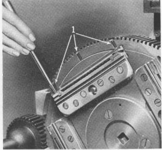
FIG. 34-1. View of method of changing mold liners.
