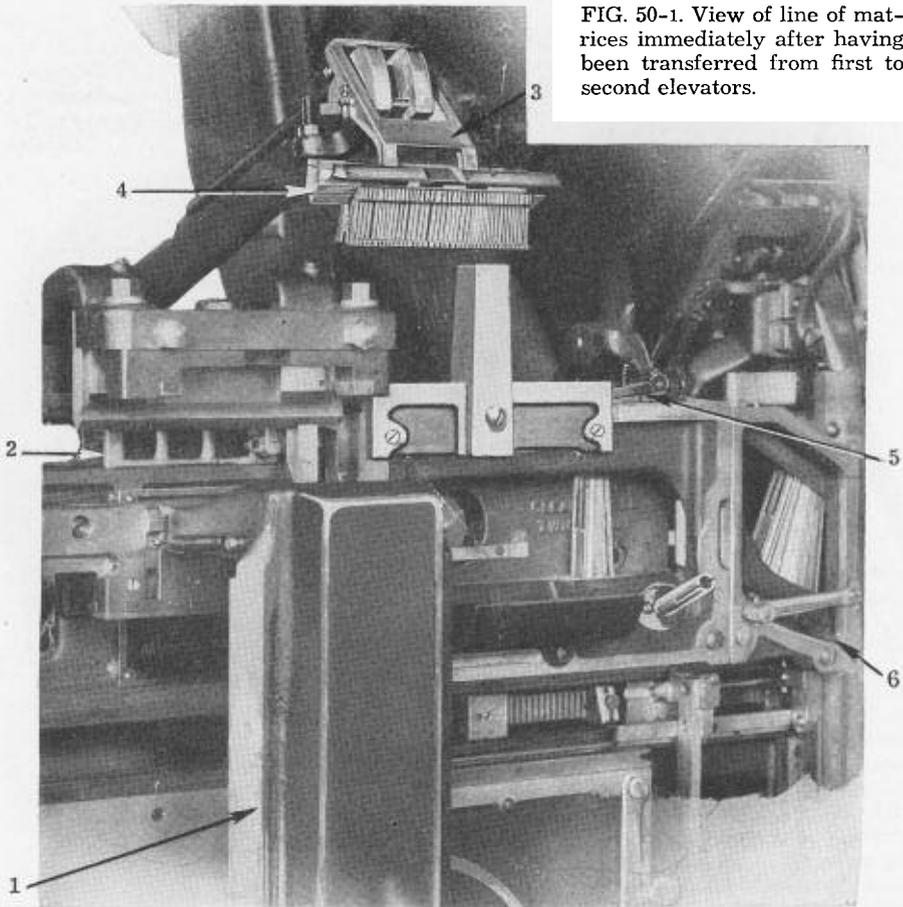
FIG. 50-1. View of line of matrices immediately after having been transferred from first to second elevators.
