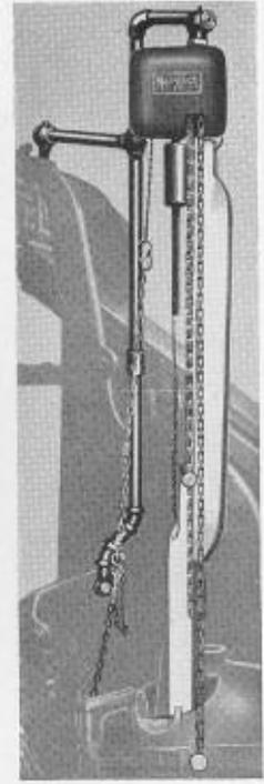
FIG. 42-1. Gas pot with metal feeder.
