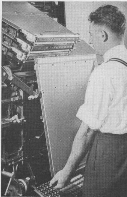
FIG. 61-1. Illustration showing method of changing magazines.
