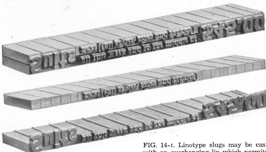
FIG. 14-1. Linotype slugs may be cast with an overhanging lip which permits large characters to lap over one or more adjacent slugs. The upper section of this illustration shows such a combination, and the lower, the two slugs separated. The mold in which they are cast is shown in Fig. 33-1.
