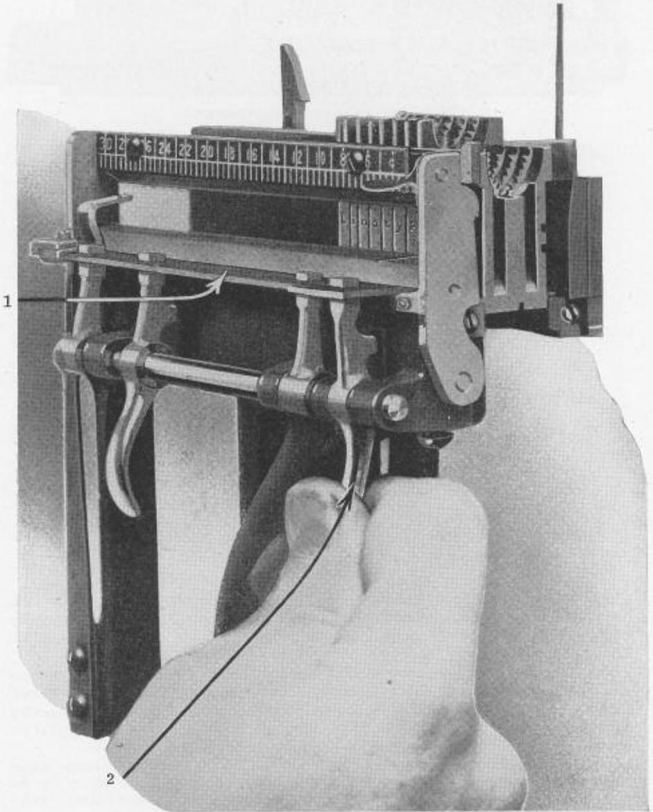
FIG. 26-1. This view indicates aligning and casting level. Assembled in this manner top characters of the lower matrices and bottom characters of the raised matrices will be cast in the same line.
