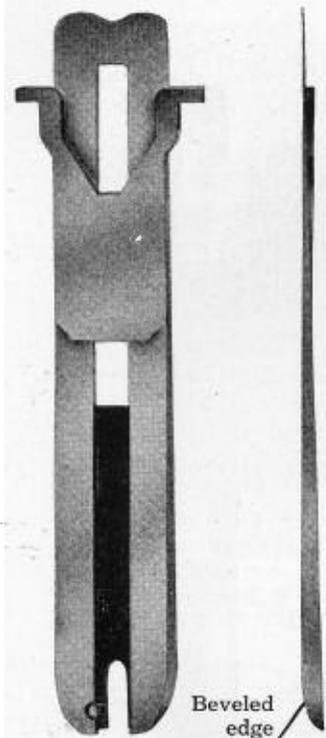
FIG. 7-1. Front and side views of the Linotype spaceband.
