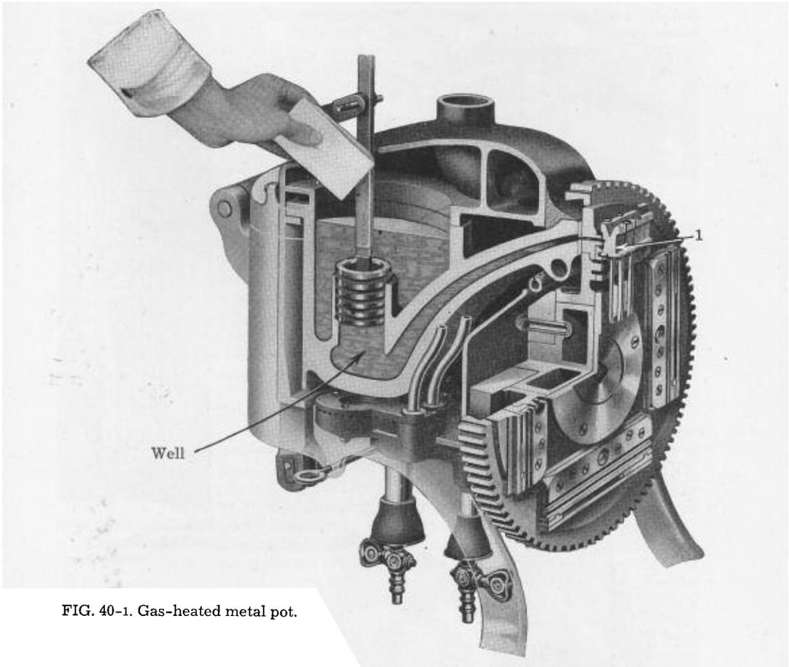
FIG. 40-1. Gas-heated metal pot.
