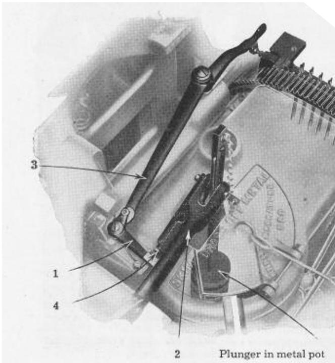
FIG. 43-1. The pot pump stop. Arm 1, which locks the pump lever 2, does not move back and allow pump lever to descend unless the front part of operating lever 3 is pressed to the right by a completely filled line of matrices and spacebands. If arm 1 has not moved back, catch block 4 on pump lever comes in contact with arm 1 and keeps the pump lever from descending.
