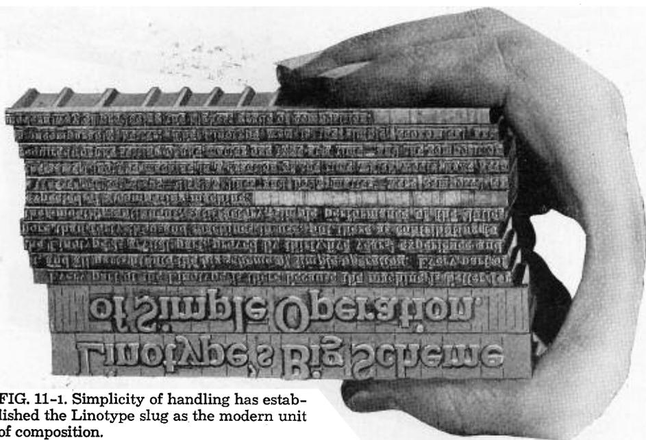
FIG. 11-1. Simplicity of handling has established the Linotype slug as the modern unit of composition.
