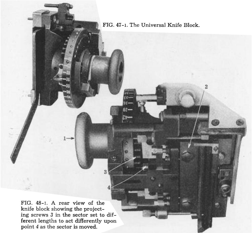
FIG. 48-1. A rear view of the knife block showing the projecting screws 3 in the sector set to different lengths to act differently upon point 4 as the sector is moved.
