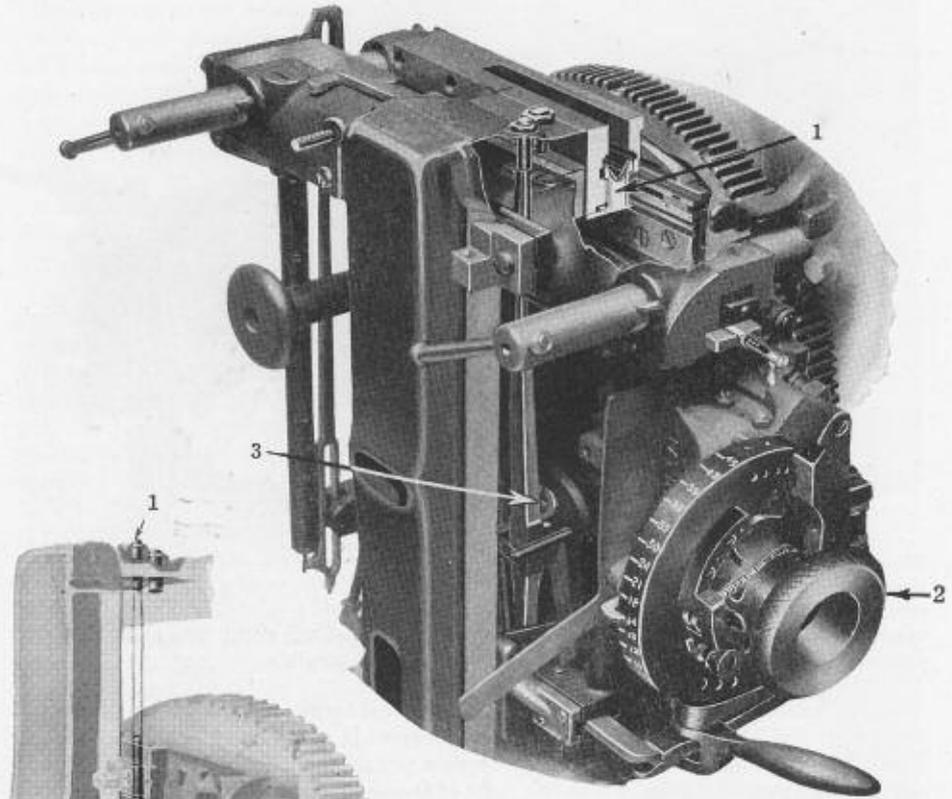
FIG. 38-1. Another view of the first elevator, this time from the right-hand side. It shows the position of the first elevator at the time of casting.
