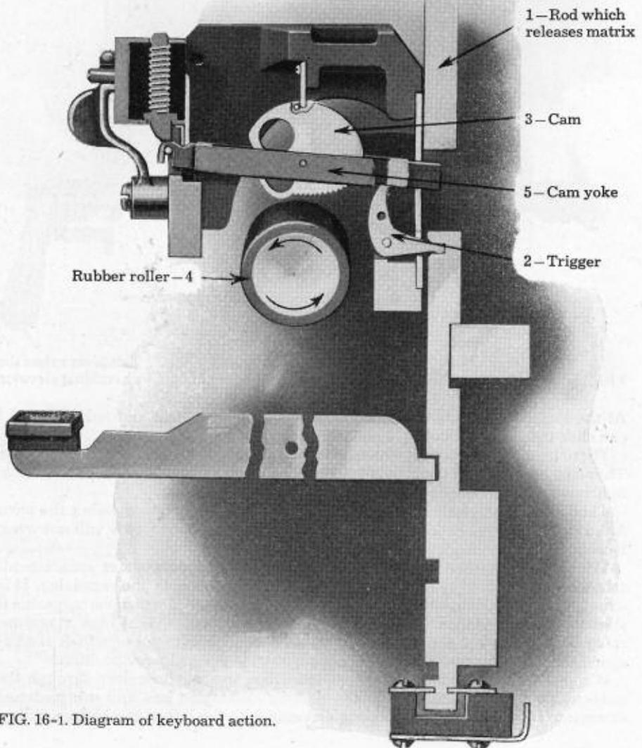
FIG. 16-1. Diagram of keyboard action.
