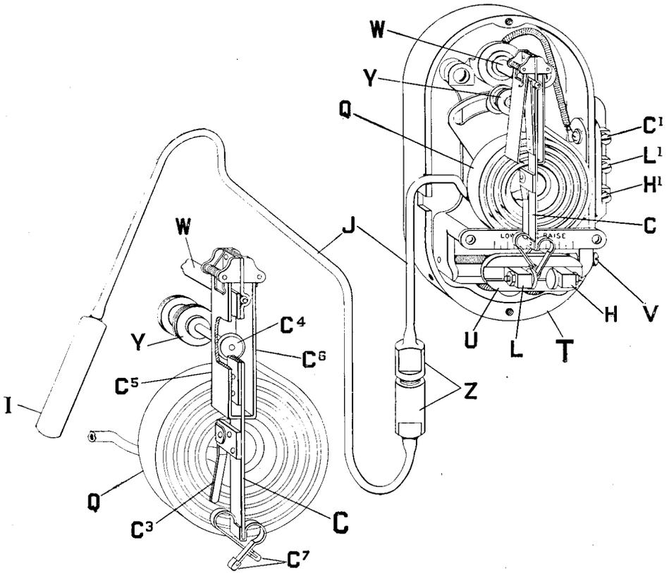
*Dynamic Thermometer Cover Removed, Fig. 3*
