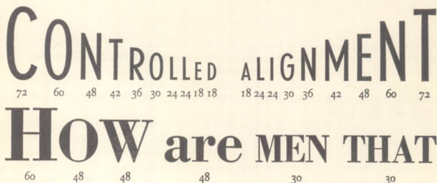
FIG. 14-36. Controlled Alignment. The upper line is an extreme demonstration showing how the base alignment of A-P-L matrices makes display combinations quite automatic. The lower line shows how this simple combination of sizes provides a new economy in display. Hitherto such combined types had to be aligned by slow hand work. Figures below the characters indicate point sizes.
