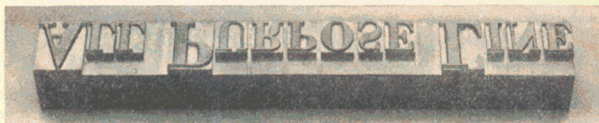
FIG. 22-36. Raised initial arrangement cast on A-P-L.
