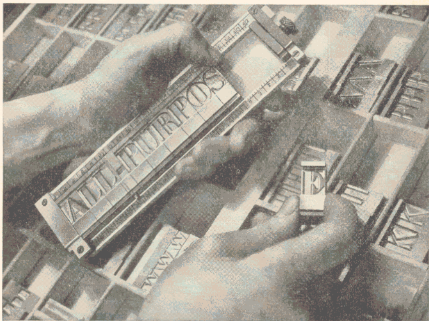
FIG. 8-36. Illustration of the method of composing a line of A-P-L matrices.
