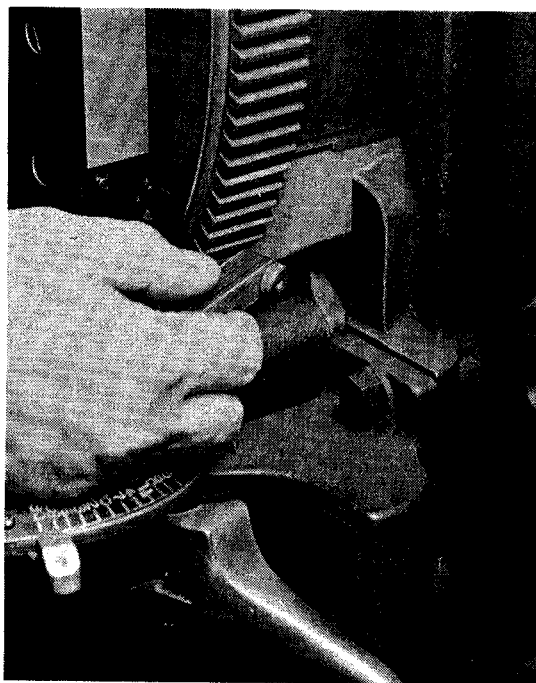
Figure 3. This adjustment helps to remove “slop” in the slide as it moves forward to lock-up.
